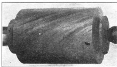
Fig. 137. Gavel Roughed to Shape.
