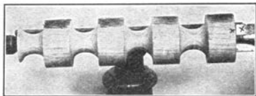
Fig. 52. Bead and Cove, Coves Completed.
