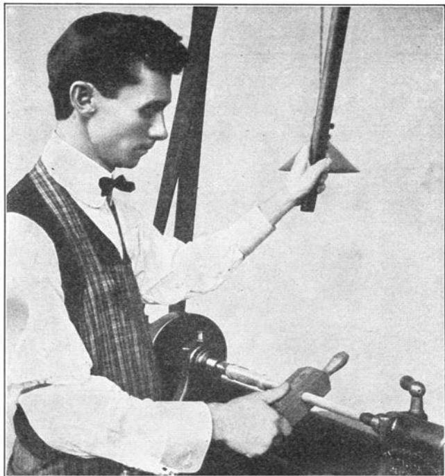
Fig. 184. Cutting the Threads for a Wooden Screw.
