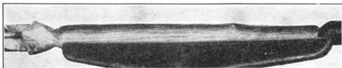
Fig. 141. Handle Roughed Out.
