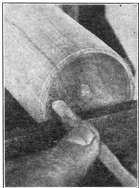
Fig. 102. Smoothing Inside of Box Cover.
