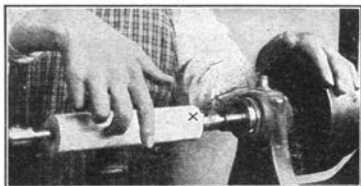
Fig. 10. Stopping the Lathe and Testing the Surface.
